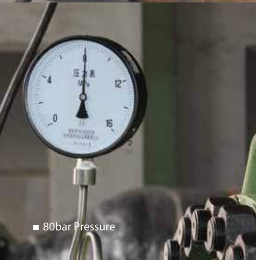
■ Pressure Test Of Discharge Hose
